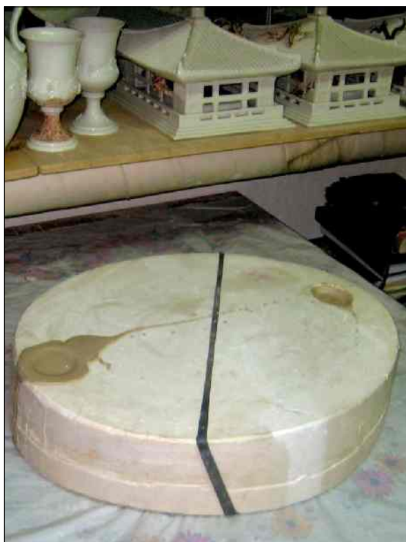
Fig. 1. Mould with two funnel-shaped holes.
