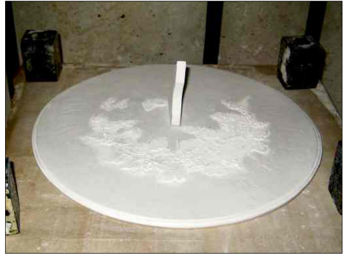
Fig. 9. The enamelled dial is ready for firing in a kiln.
