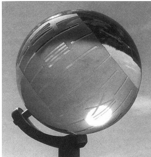
Fig. 1: The "sun circle" covers the hour lines 12h (&XII) and 11h (I) equally: the current time lies in between, thus 11:30 h.
